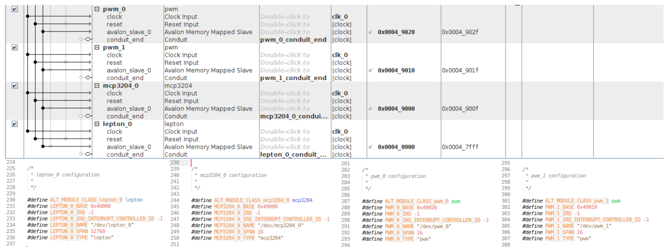
Figure 1: At the top, the QSys editor. At the bottom, the system.h file that was automatically generated. It can be seen that the memory mapping was taken by QSys.
