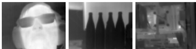
Figure 2: The images that we captured using the thermal camera. From left to right: Face with glasses, Glass Bottles, Inside a Computer with CPU and GPU (where we can see on the left a column of chokes and capacitors and on the right a crystal both of them being a major source of heat. We can also see on the bottom right an SSD).
